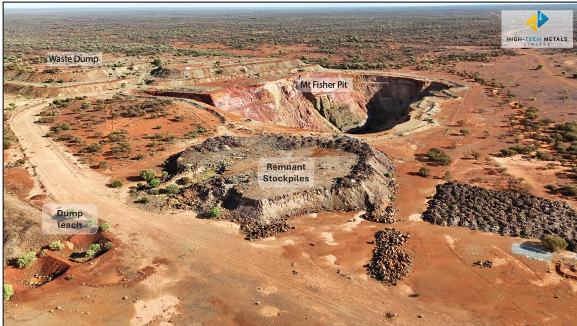
Figure 3: Mt Fisher Mine looking north-west showing historical pit and waste dumps. Tailings storage facility out of field of view.
