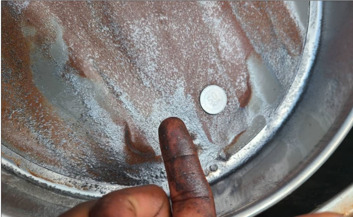
Figure 3: Image depicting disseminated flake graphite (0.47%) with metallic grey lustre and streaks, hosted in a ferruginous clay matrix within the mottled zone (ALAAU001, 9–10 m), observed during desliming.
