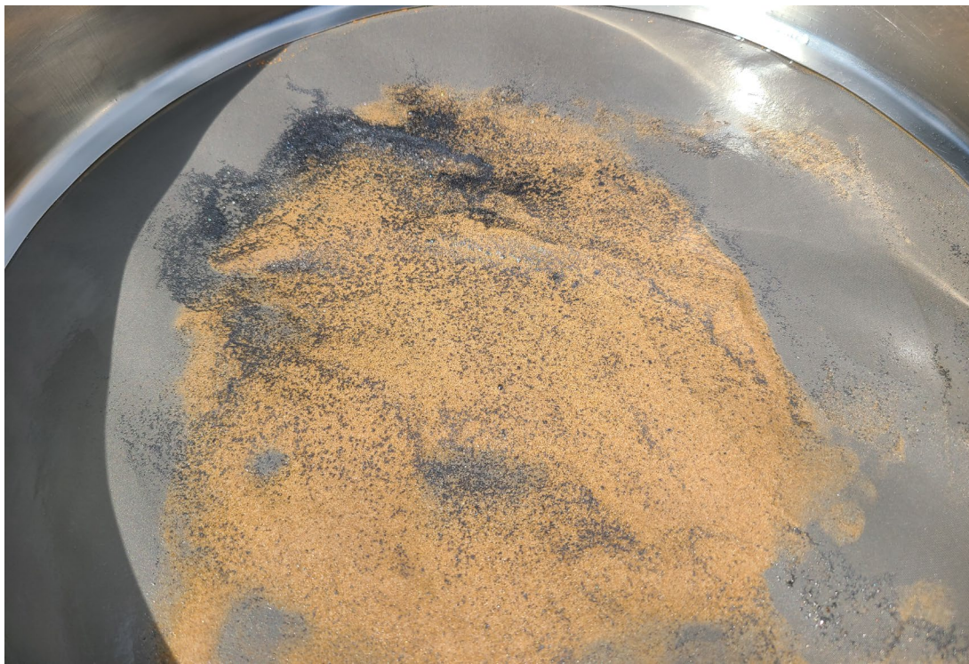
Figure 2: Image depicting disseminated flake graphite (0.6%) with metallic grey lustre and streaks, hosted in a ferruginous clay matrix within the mottled zone (ALAAU004, 8–9 m), observed during desliming.
