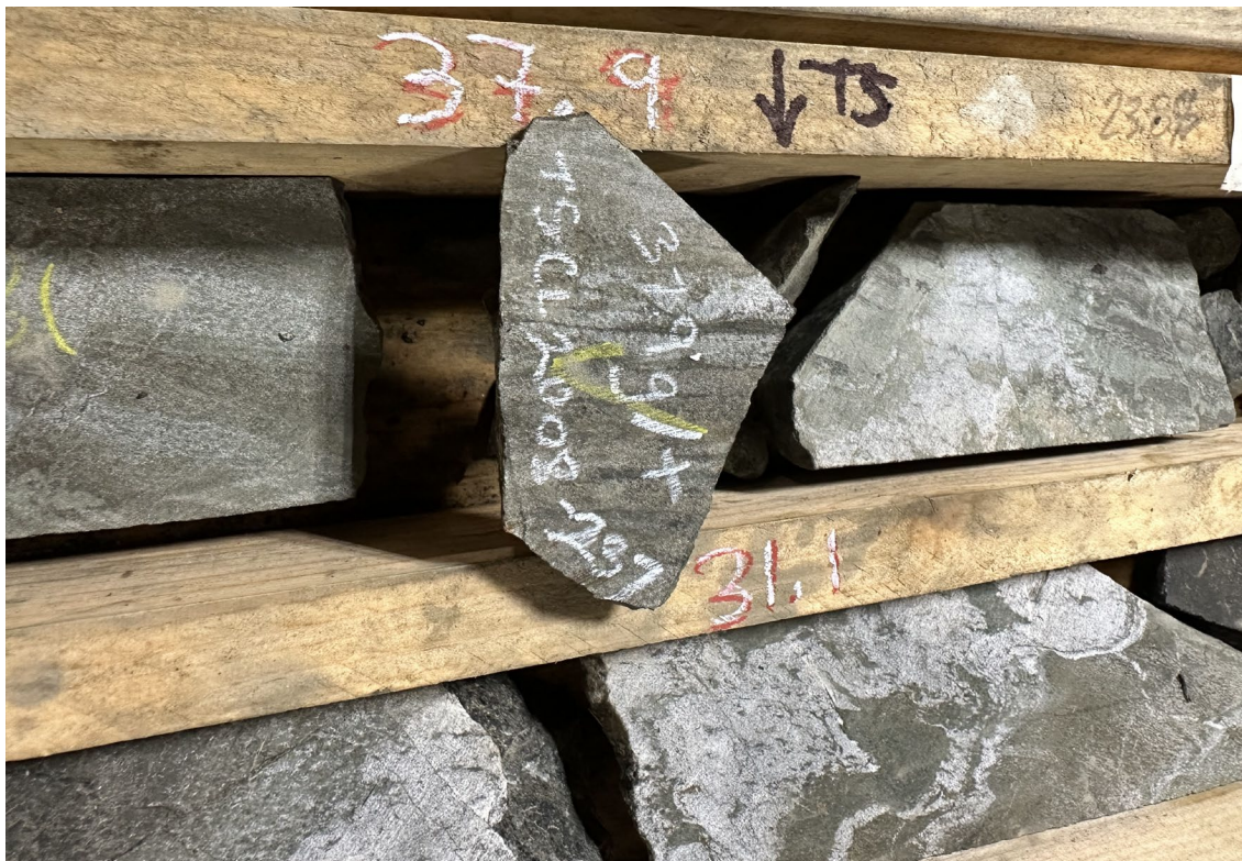
Figure 3: Section of historic core from the Arrow Zone CL-20-08 containing the intercept of 31.9 m @ 13.66 g/t Au from 17.5 m
