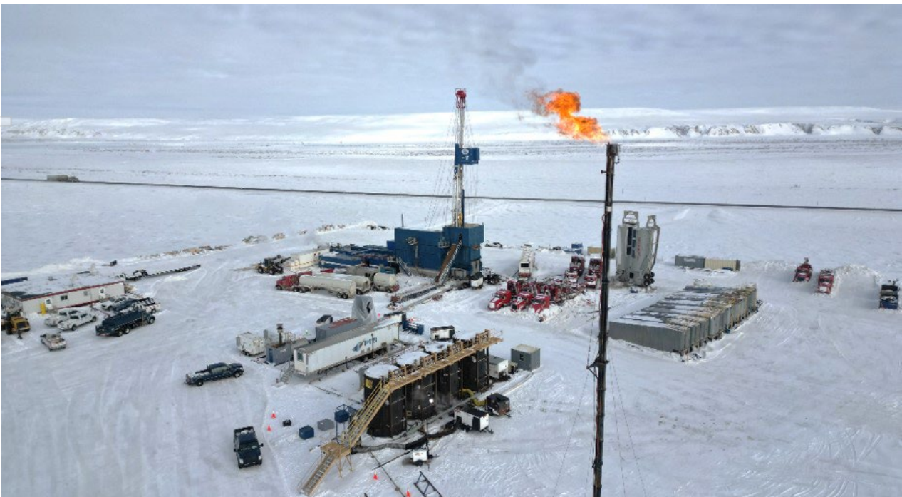
Figure 3: Project Phoenix oil flowed to surface during Hickory-1 flow testing operations Q1 2024.
