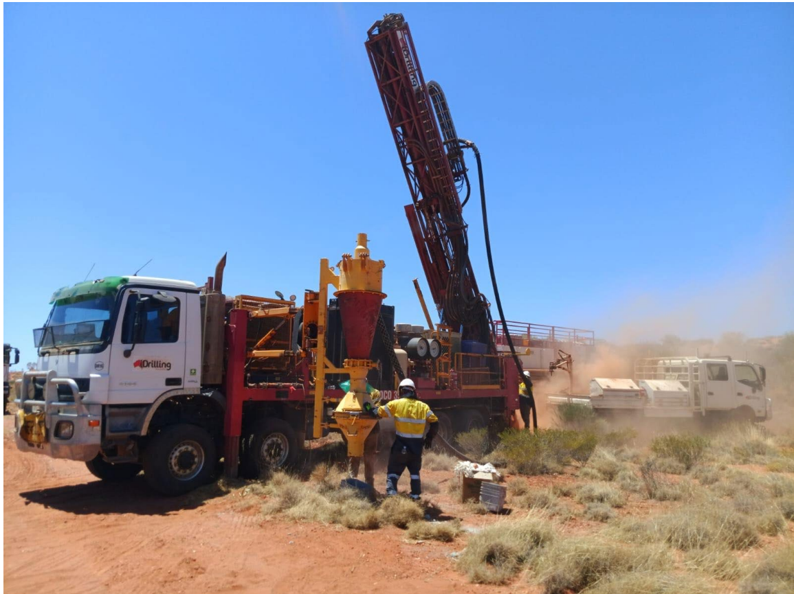
Figure 1: RC rig drilling at the Grace Gold Project
