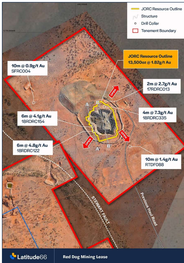
Figure 2: Plan view of Red Dog granted Mining Leases showing historically mined open pit, previous haul road, drill collars and location of long section A-A' (Figure 3) and oblique cross section B-B' (Figure 5)
