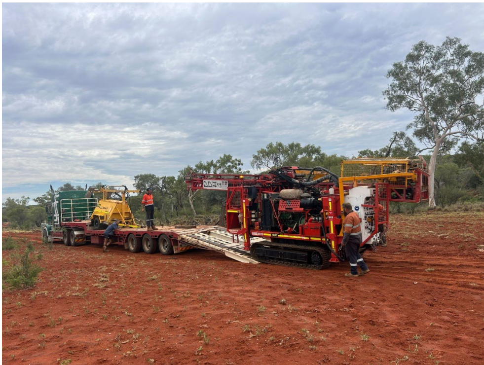
Image 2: Track mounted diamond drill rig arriving in central Australia from the Speewah Fluorite Project
