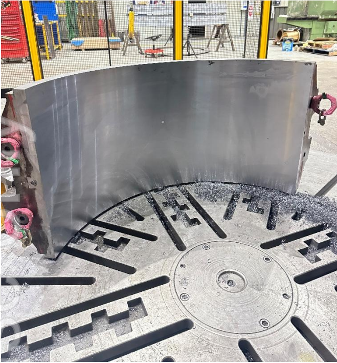
Figure 5a: Bearing white metal reline
