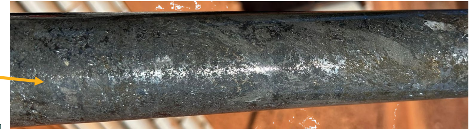
Core from drillhole EHDD25001 (~240m depth) showing semi-massive sulphide mineralisation (pyrite-pyrrothite-boulangerite ( Pb_5Sb_4S_{11} ))
