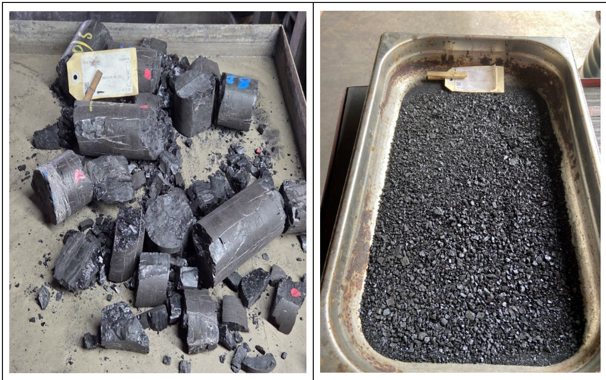
FIGURE 2: SAMPLE QB02 (“D” SEAM) 63MM CORE FROM RSC015C A & CF1.40 PRODUCT COAL
