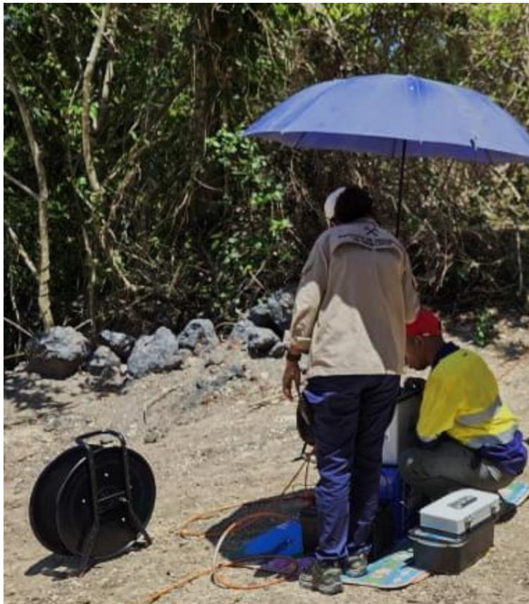
Figure 2: Deployment of Res-IP electrodes at Ira Miri
