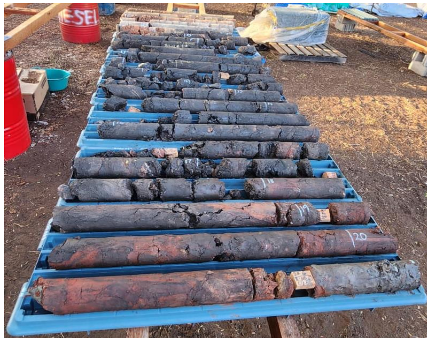
Figure 5: Manganese oxides in core from EMDD033, For visual estimates and visual estimates disclaimer please refer to table 1
