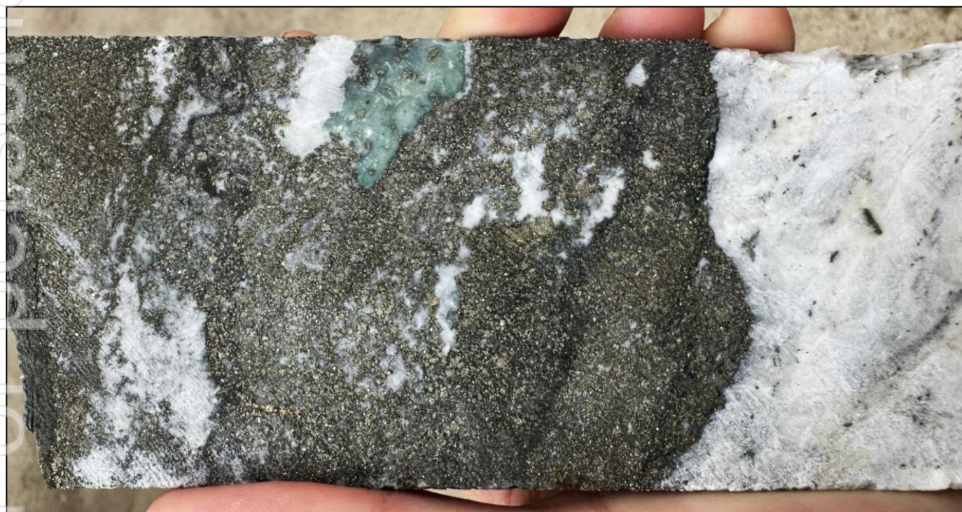
Figure 5. Core photograph of ZRSD25206 from 347.3m to 348m of cement-supported polymictic (andesite, limestone) breccia with disseminated to semi-massive pyrite –13.5g/t Au.
