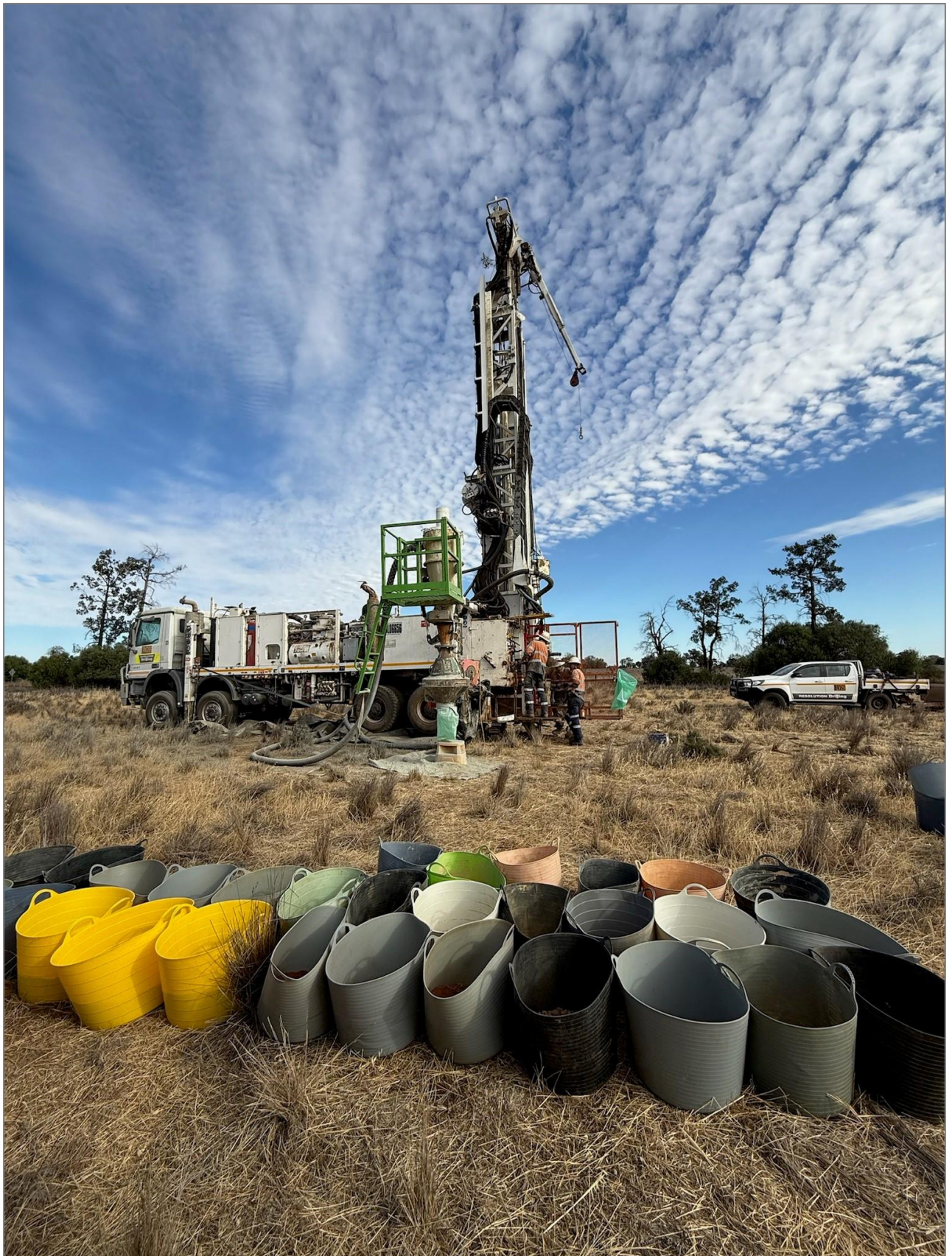
Figure 1: Air core drilling rig operating at the Murga Exploration Target November 2025.
