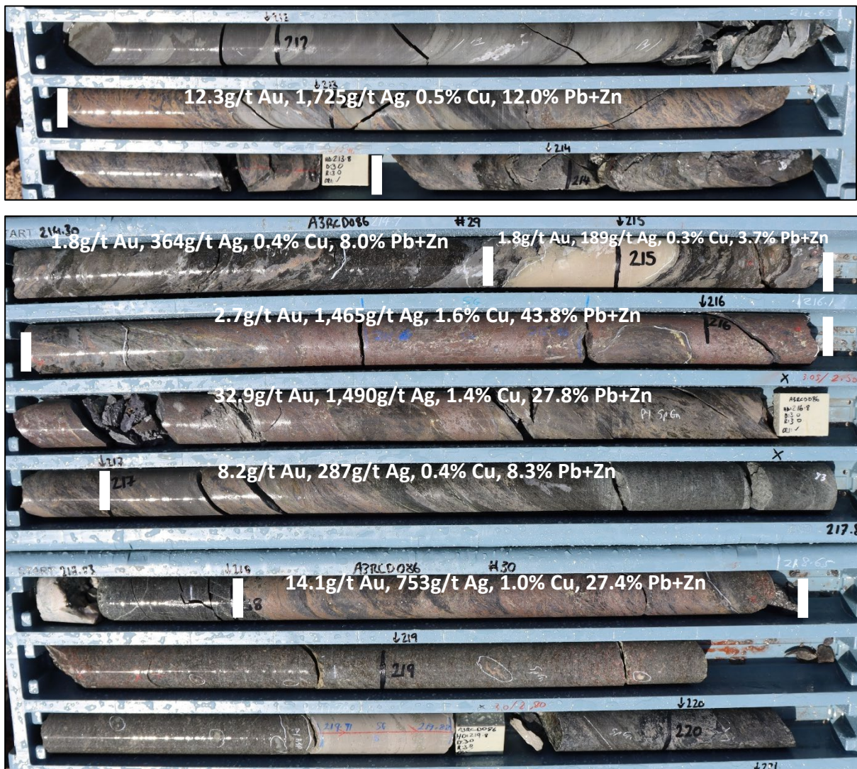
Figure 2: Core photographs of the gold-silver bearing massive sulphide zone in A3RCD086 grading 6m at 11.0g/t Au, 942g/t Ag, 0.8% Cu & 17.9% Pb+Zn; 2,474g/t AgEq from 212.65m.
