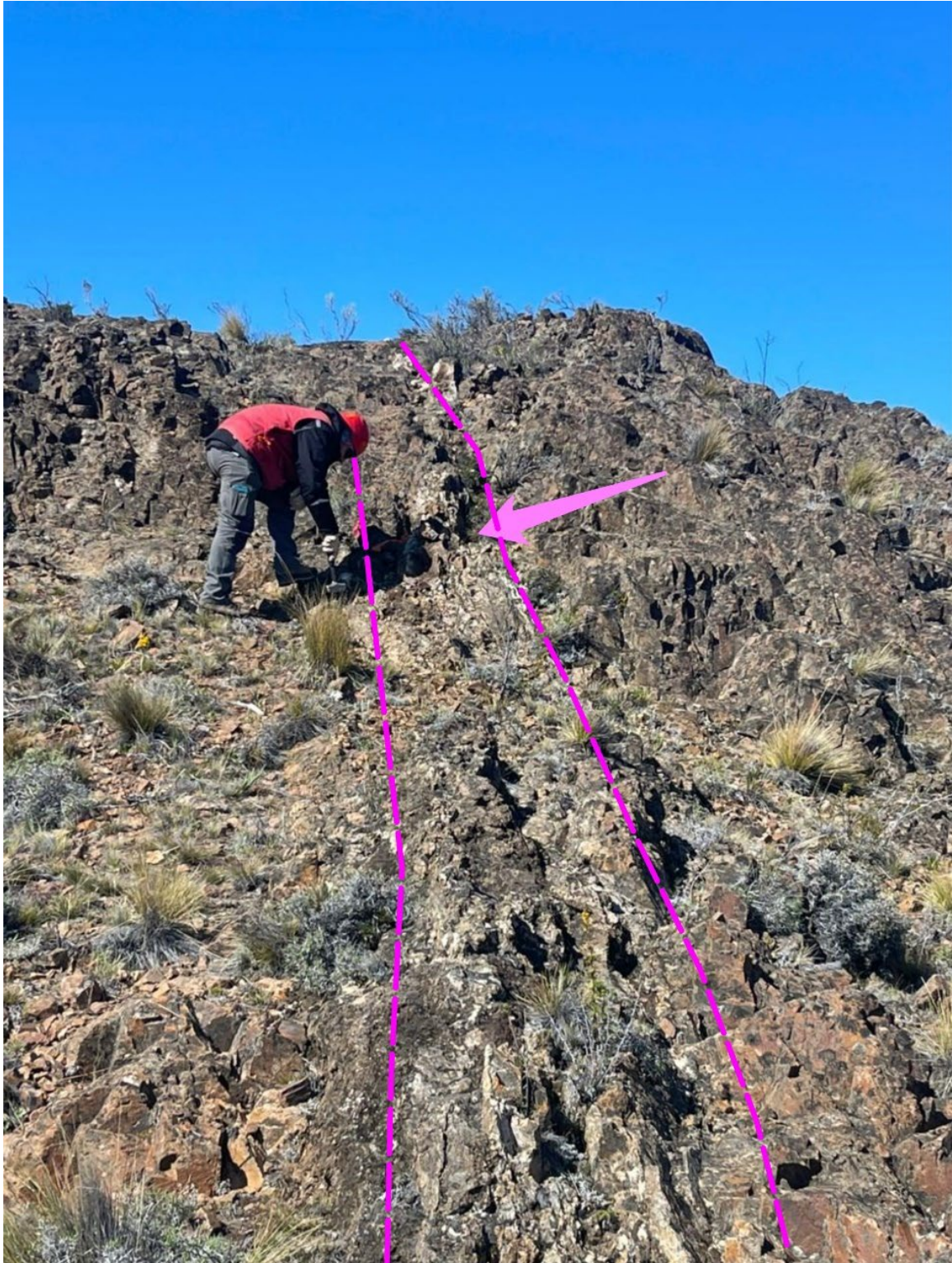
Figure 3. Typical vein outcrop observed within the Taitao East project area. Pink arrow indicates location of Sample ID 45408 returning 2,935g/t AgEq (528g/t Ag & 29g/t Au or 35.4g/t AuEq).
