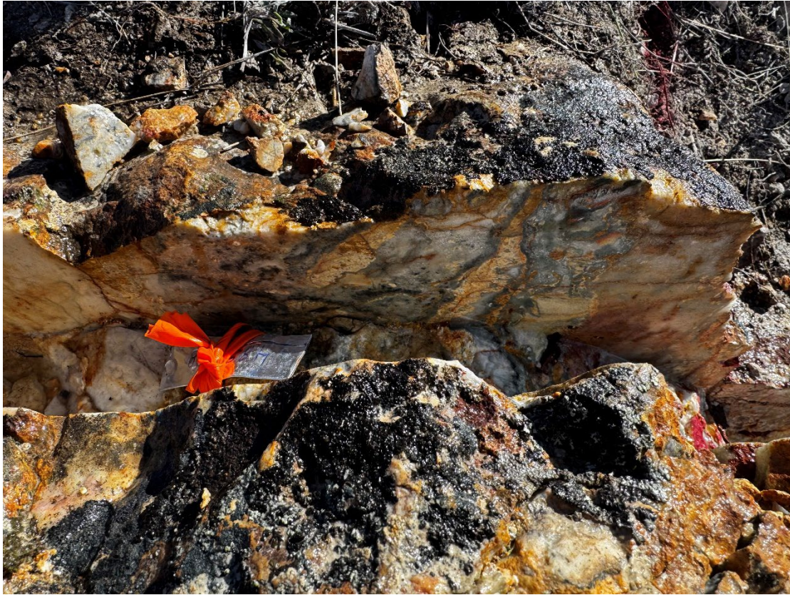
Figure 6. Sawn Channel sample showing epithermal textures within the vein. Sample ID CC278, returning 1.6m @ 333g/t AgEq (136g/t Ag & 2.4g/t Au) or 4.0g/t AuEq. Looking North.
