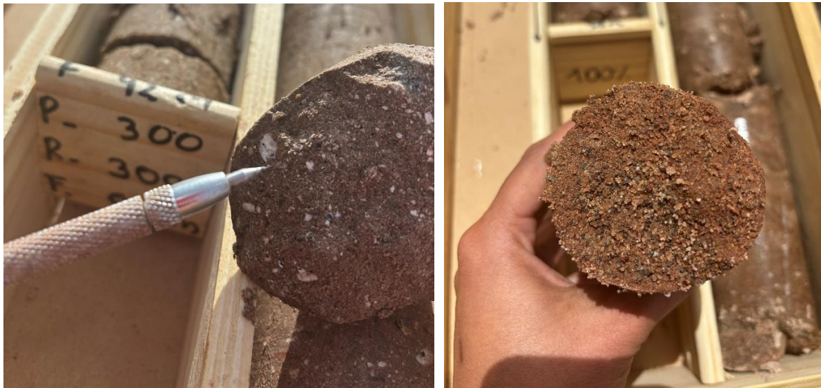
Figure 4. Core- fine sandstone clasts and gypsum crystals and RHS showing porous sandy clast 92-98m
