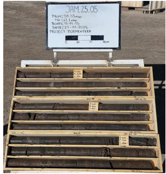
Figure 5. Core trays showing sandy lithologies from black (67m) to brown sandstones (from 70m).
