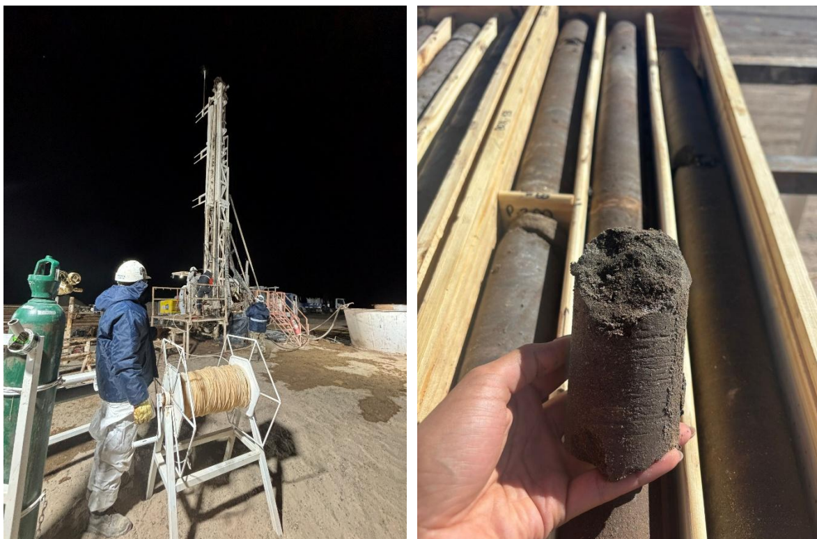
Figure 2. Packer test operating and right hand side picture shows porous core with sand evident.
