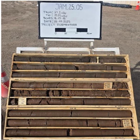
Figure 5. Core trays showing sandy lithologies from black (67m) to brown sandstones (from 70m).
