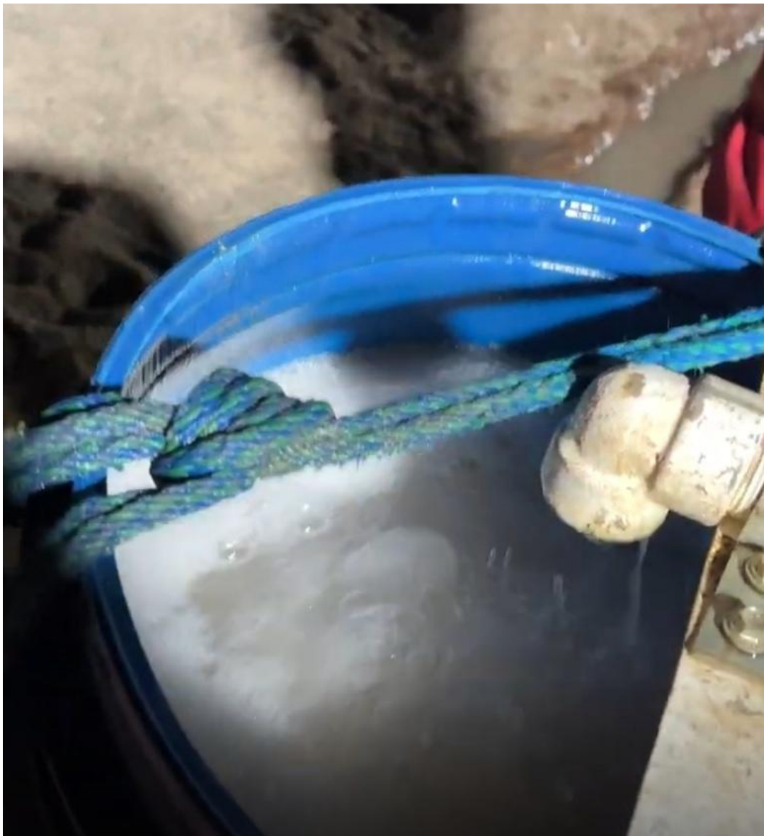
Figure 1. Brine filling into the 150L drum at 1286L/per hour.
