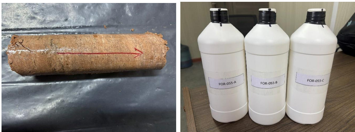
Figure 3. Core prepared for porosity testing and bottles sealed with QA/QC chain of control for laboratory analysis
