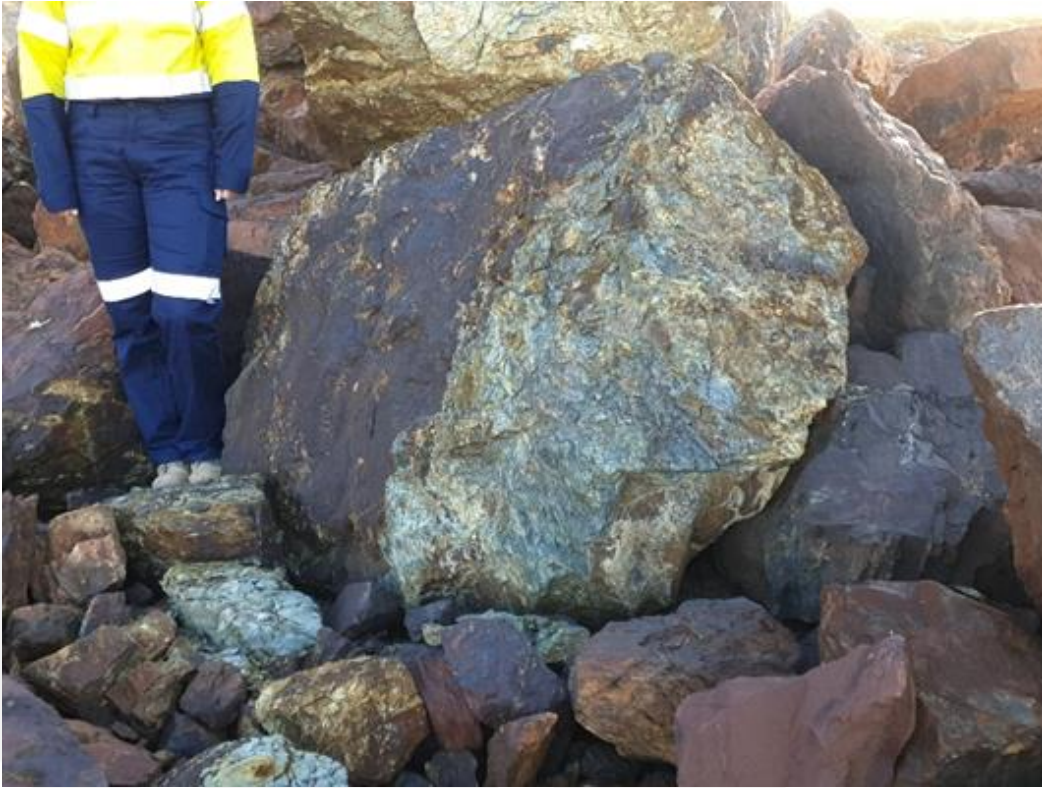
Figure 4: Oversized transitional high-grade ore from Mt Fisher low-grade stockpile (sample MFS007: 14.75 g/t Au).
