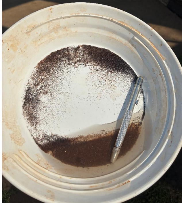
Figure 2. Rutile in a panned heavy mineral concentrate (HMC) from soil sample SS118 at Mkanda Rutile Project. The soil sample was taken from surface and panned to a concentrate for mineral identification. Final Assay results returned from Scientific Services was 1.11% rutile 1 .
