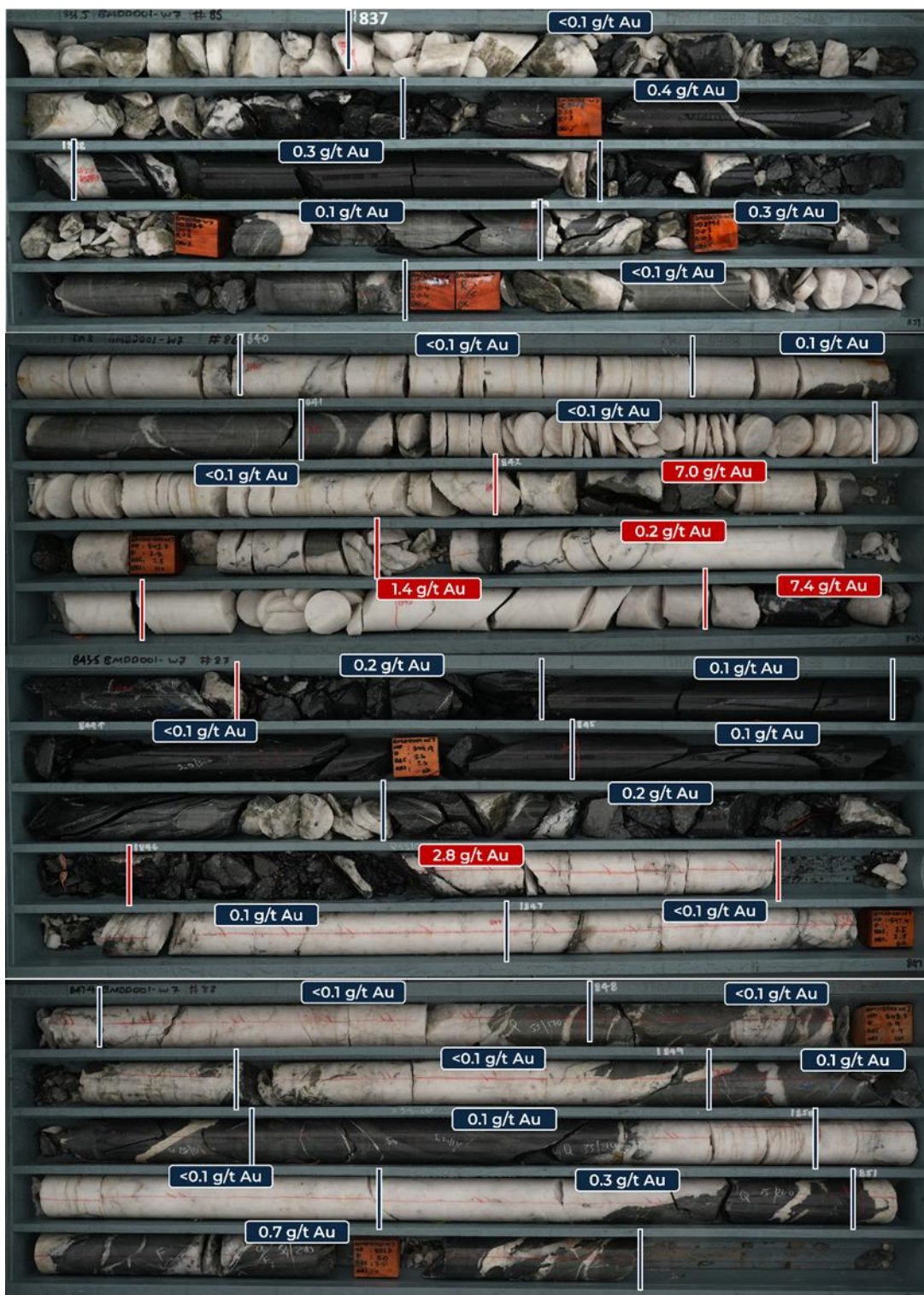
Figure 12 Zone of mineralised quartz in BMDD001W7 from 836.5-851.7m with significant intercepts in red
