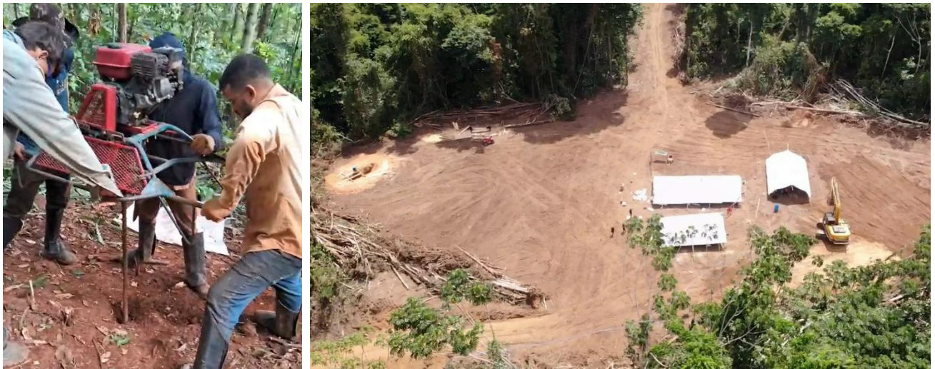
Figure 5: Left – Mechanised auger operating on South Oko. Right – Preliminary setup of permanent camp commencing at South Oko, ahead of 2026 drill program
