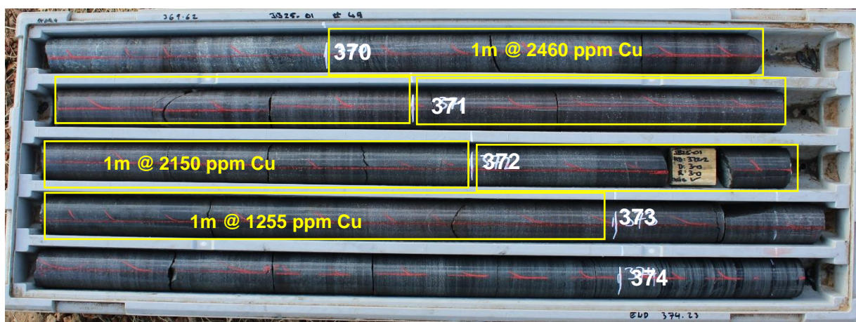
Figure 5 – Tray 49 from JB25-01 showing intervals containing elevated Cu from 370m downhole.
