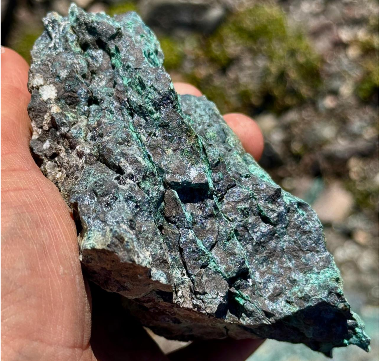
Figure 4 - Photograph of sample X961221 which returned 37.4% Cu and 72.9g/t Ag . Photo depicts vesicles infilled by chalcocite and secondary malachite tracing fractures through the mineralised flow top basalt.
