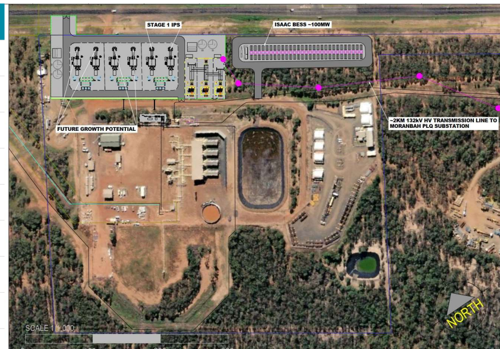
Layout: The IPS will be located on QPM owned land 2km from Powerlink's Moranbah 132kV substation
