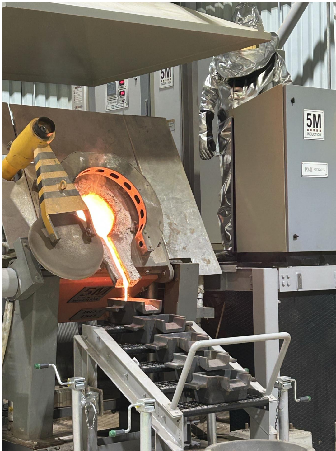
Figure 2: In the gold room- the first doré pour from the Tavşan gold-silver mine.
