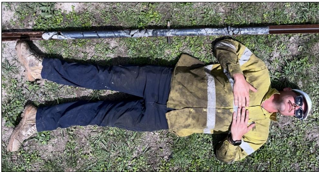
Figure 1 : DTM driller and 1.6m of the 2.2m section of CBADD010 where massive stibnite and quartz veining with stibnite was intersected. A small (20cm) fault zone is also present in this interval. *
