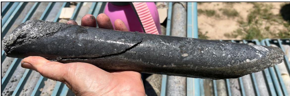
Figure 5: 0.3m of quartz hosted massive stibnite* in hole CBADD007 from 139m. Fault gouge seen on the left of hand specimen, indicating the fault controlled nature of mineralisation at Coonambula. *
