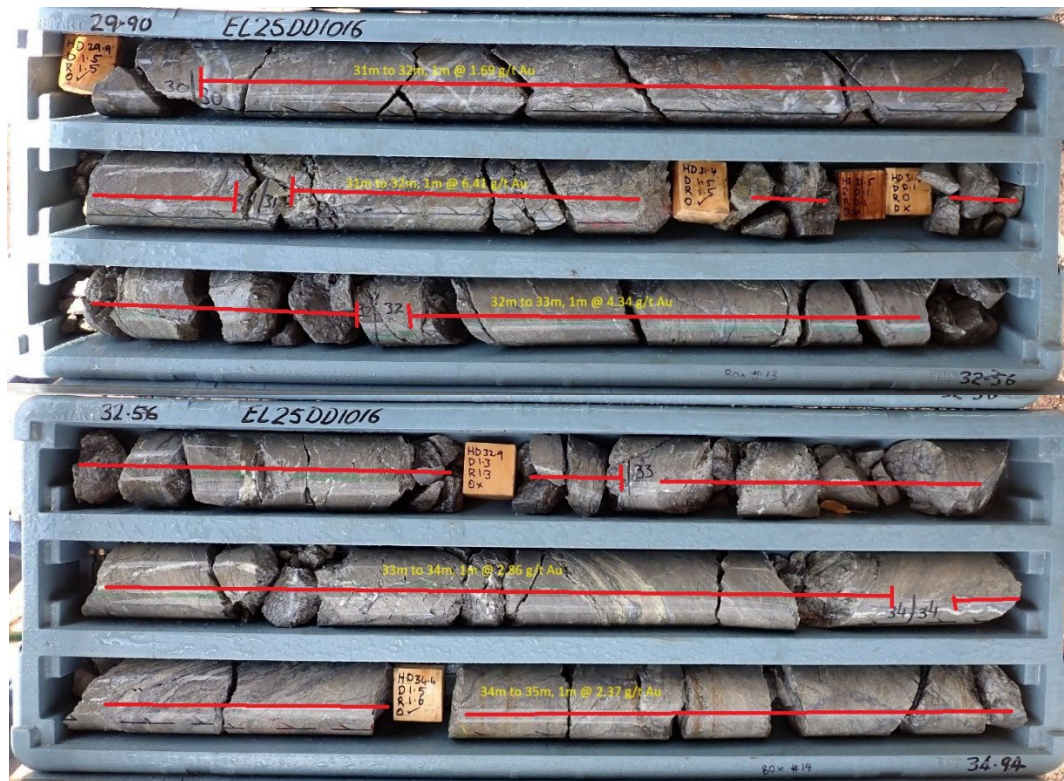
Figure 3: Electric Light diamond drill core from 29.90m to 34.94m, 5.04m @ 3.53 g/t Au
