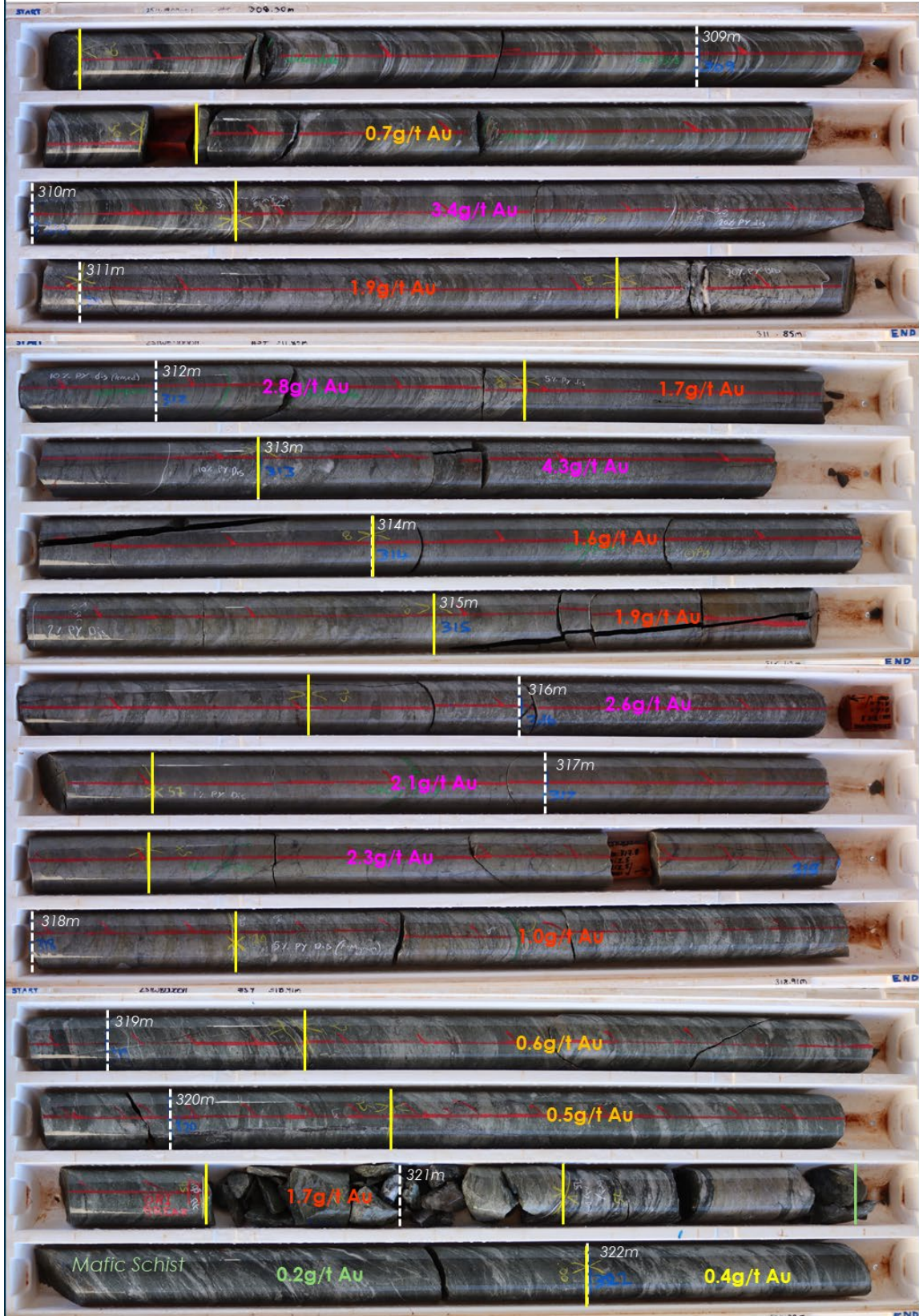
Figure 3: HQ diamond core from 25IWBD0011 showing the mineralisation intercepted that includes 7.95m @ 2.5g/t Au from 310.25m. Metre marks are shown and annotated in white; sample boundaries are marked in yellow.
