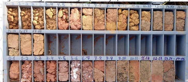
Figure 5A: Auger drill cutting chip library of CDE-AD-0002 auger hole
