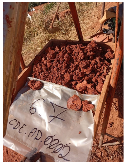
Figure 6: Kamafugite red saprolite sample from drill run in CODA East-CDE-AD-0002
