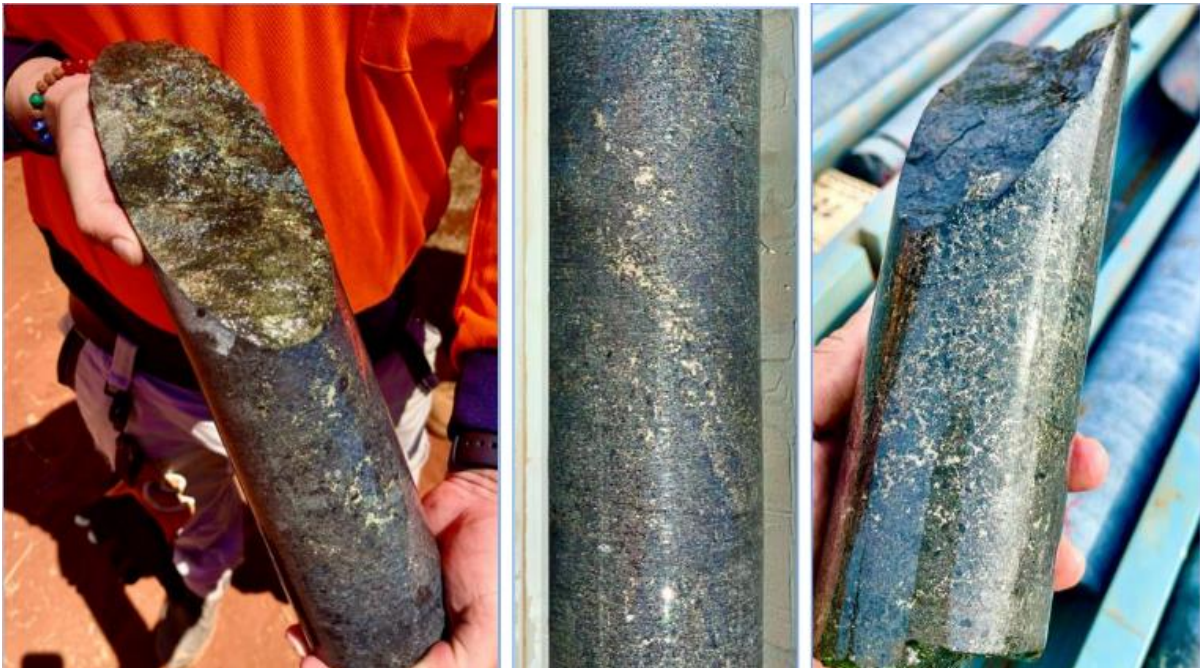
Figure 1. (Left to right) Chalcopyrite-rich fracture-fill vein and adjacent net-textured to globular sulfide mineralisation in drillhole SWDD003 (75.38–75.80 m); disseminated chalcopyrite–pyrrhotite–pentlandite sulfides in SWDD003 (200.1–200.6m); and net-textured magmatic sulfides in SWDD002 (110.3–110.7m). Assays pending. Refer to ASX announcement dated 29 October 2025 for further details regarding SWDD002 and SWDD003 visual estimates.
