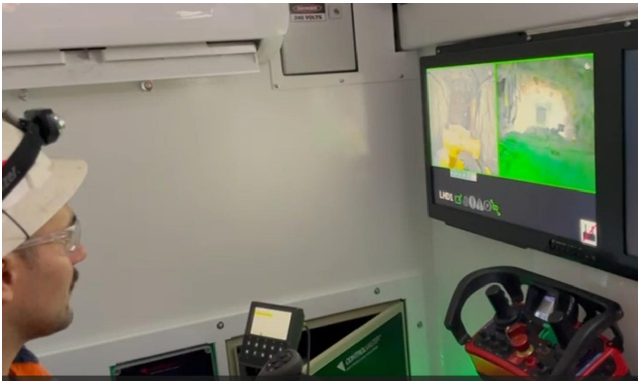
Figure 1 Tele remote specialist bogging out the first ore with the Aramine loader in the 1438 North stope.
