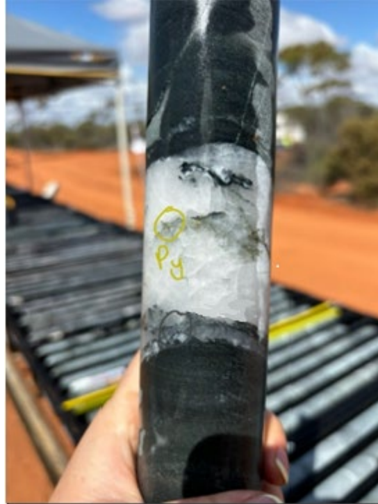
Figure 6: SMXDD003 – quartz, pyrite, pyrrhotite, graphite vein at 830m. No significant results returned
