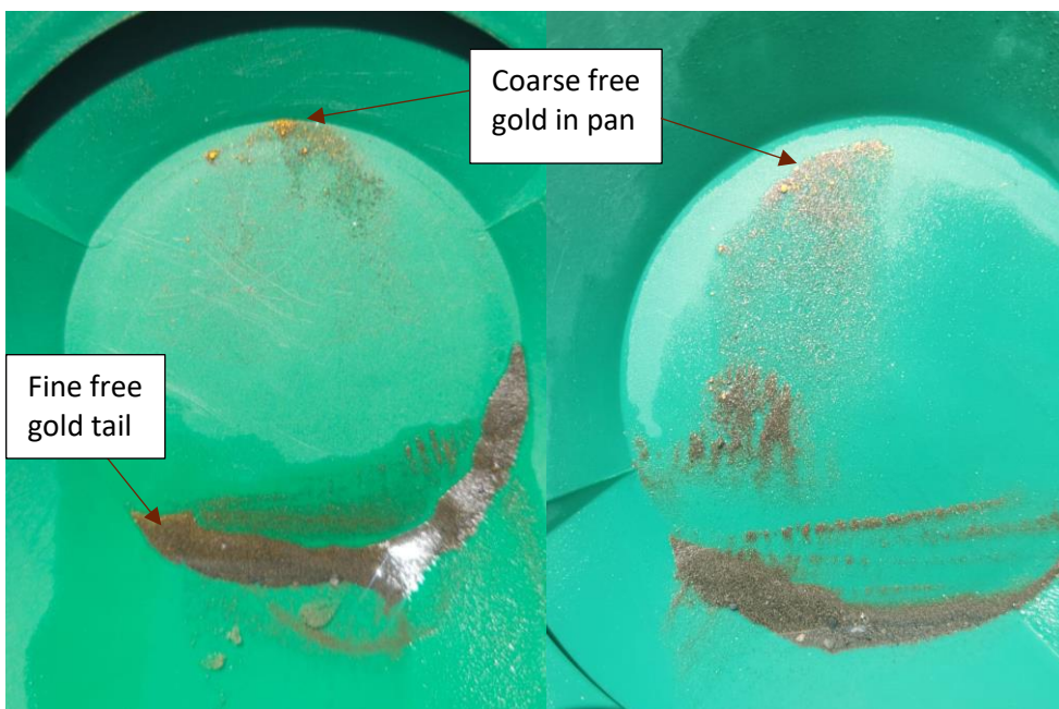
Figure 5. Spring Creek Prospect – Free Coarse Gold in Pan from SCRC016 interval 15 – 16m – 1.0m at 58.3g/t Au
