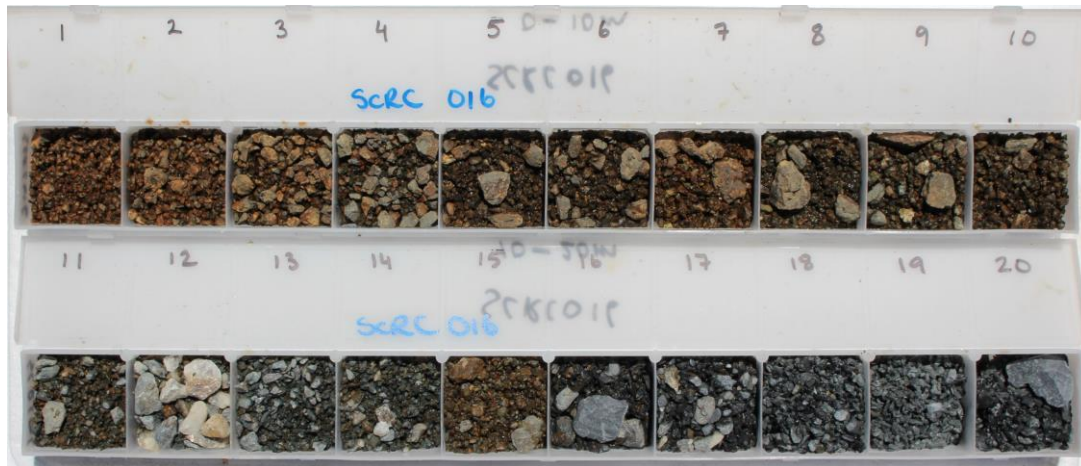
Figure 6. Spring Creek Prospect – RC Drill Chips SCRC016 0 – 20m – mineralised interval 6.0m at 9.99g/t Au from 11m to 17m
