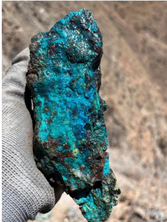
Figure 4: LHS: Cinto surface grab sample 17142 with visible copper oxides and silicification returned 7.14% Cu RHS: Grab sample 17181 (1.0 % Cu) with copper oxides and hyaline quartz from outcrop 7
