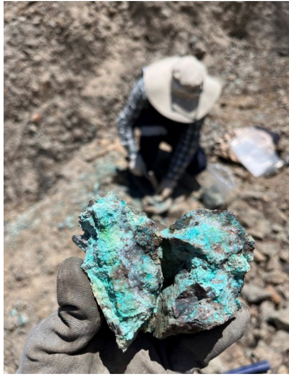
Figure 4: LHS: Cinto surface grab sample 17142 with visible copper oxides and silicification returned 7.14% Cu RHS: Grab sample 17181 (1.0 % Cu) with copper oxides and hyaline quartz from outcrop 7
