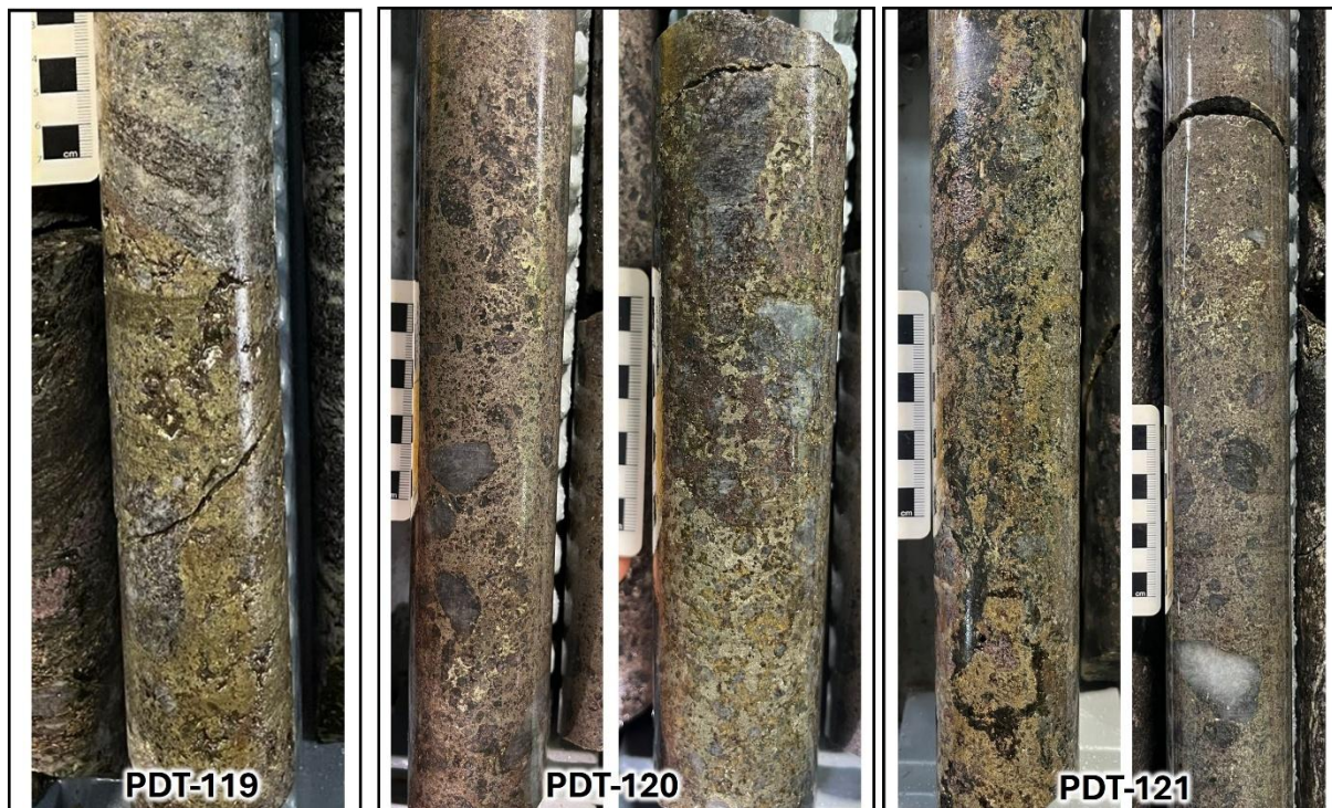
Figure 1: Mineralised intervals at Touro Prospect-recent drilling. From left to right: PDT-119 from 65.5m downhole; PDT-120 from 66.25m (visual estimate of 8% chalcopyrite and 12% sphalerite) and 69.2m (visual estimate of 1% chalcopyrite and 25% sphalerite); PDT-121 from 95m and 101.85m (Visual estimate of 3% chalcopyrite + 1% sphalerite, and 10% chalcopyrite + 5% sphalerite, respectively). Depth refers to base of core in photo. Dark brown mineral is sphalerite (zinc sulphide), golden colour is chalcopyrite (copper sulphide), pale yellow is pyrite (iron sulphide) and bronze colour is pyrrhotite (iron sulphide).
