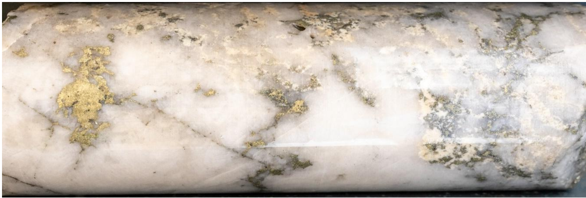
Figure 5 Magmatic quartz with blebby chalcopyrite (yellow) overprinting granodiorite porphyry at 55.8m down-hole depth in 25BRD0038. From within a 3.8m wide interval visually estimated to contain 1.5% chalcopyrite (0.50% Cu*). Core diameter 61mm.
