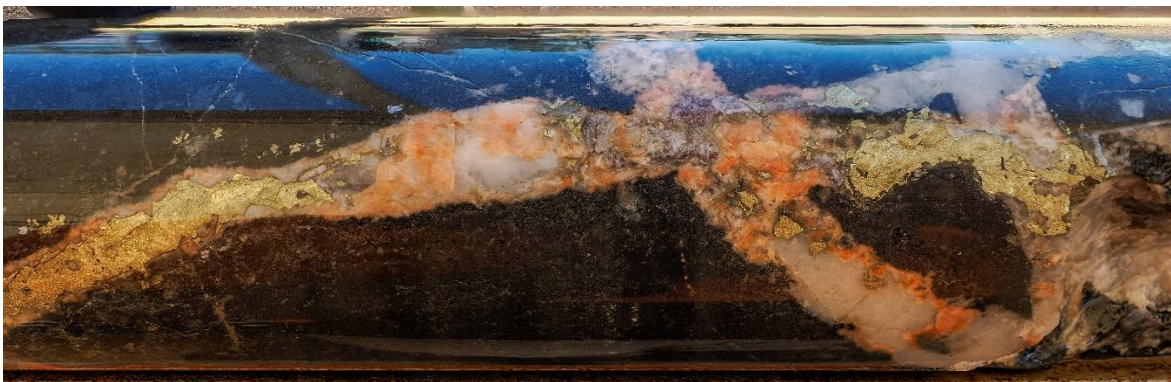
Figure 6 Multiphase quartz-feldspar-chalcopyrite-pyrite-anhydrite veins cutting volcaniclastic sediments at 336.0m down-hole depth in 25BRD0038. From within a 22.1m wide interval visually estimated to contain 0.75% chalcopyrite (0.25% Cu*). Core diameter 50mm.
