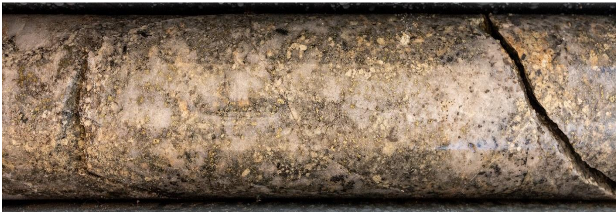
Figure 4 Altered granodiorite porphyry with silica flooding and disseminated chalcopyrite at 40.7m downhole depth in 25BRD0038. From within a 4.6m wide interval visually estimated to contain 2% chalcopyrite (0.70% Cu*). Core diameter 61mm.
