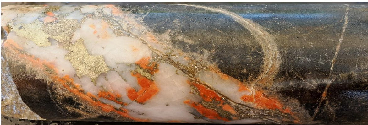
Figure 7 Coarse grained chalcopyrite (yellow) and pyrite (bronze colour) in quartz-feldspar vein cutting volcaniclastic sediments at 378.4m downhole depth 25BRD0038. From within a 14m wide interval visually estimated to contain 0.75% chalcopyrite (0.25% Cu*). Core diameter 50mm.
