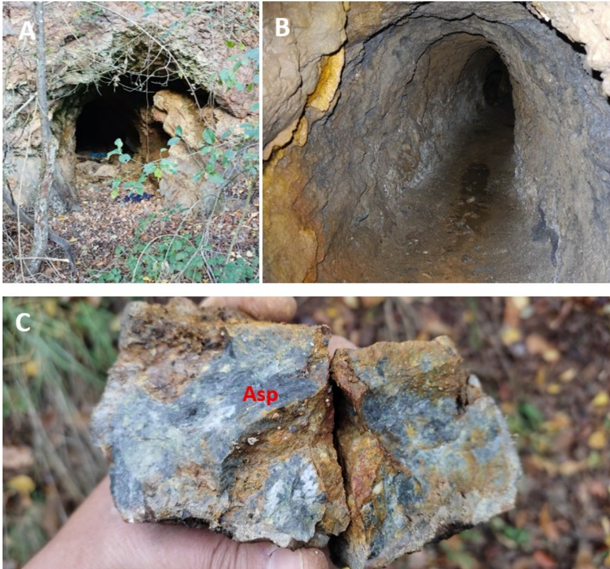
Figure 4. Mining adits in northern area of Rujak and sample from adits with arsenopyrite up to 10% visual mineral estimate. Hosted in listwanite with cockade epithermal texture. See table 3 for full table of visual estimates – expecting assay results in 8 weeks.
