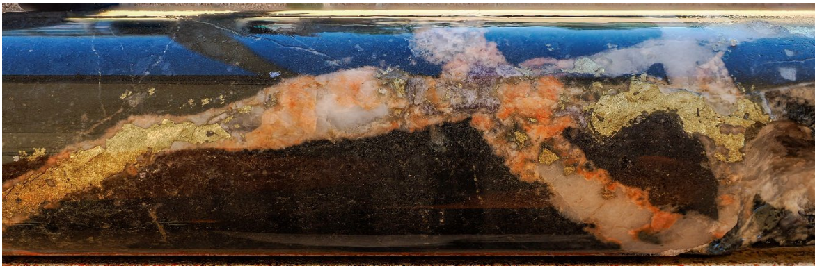
Figure 5. Multiphase quartz-feldspar-chalcopyrite-pyrite-anhydrite veins cutting volcaniclastic sediments at 336.0m down-hole depth in 25BRD0038. From within a 22.1m wide interval visually estimated to contain 0.75% chalcopyrite (0.25% Cu*). Core diameter 50mm.
