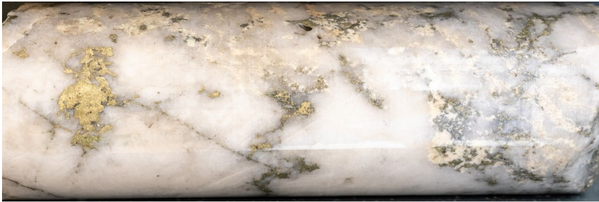
Figure 4. Magmatic quartz with blebby chalcopyrite (yellow) overprinting granodiorite porphyry at 55.8m down-hole depth in 25BRD0038. From within a 3.8m wide interval visually estimated to contain 1.5% chalcopyrite (0.50% Cu*). Core diameter 61mm.
