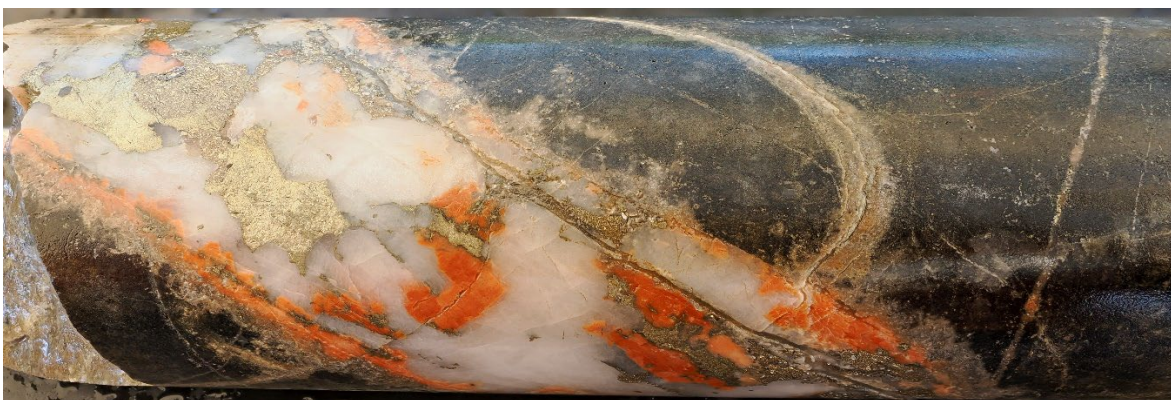
Figure 6. Coarse grained chalcopyrite (yellow) and pyrite (bronze colour) in quartz-feldspar vein cutting volcaniclastic sediments at 378.4m down-hole depth in 25BRD0038. From within a 14m wide interval visually estimated to contain 0.75% chalcopyrite (0.25% Cu*). Core diameter 50mm.
