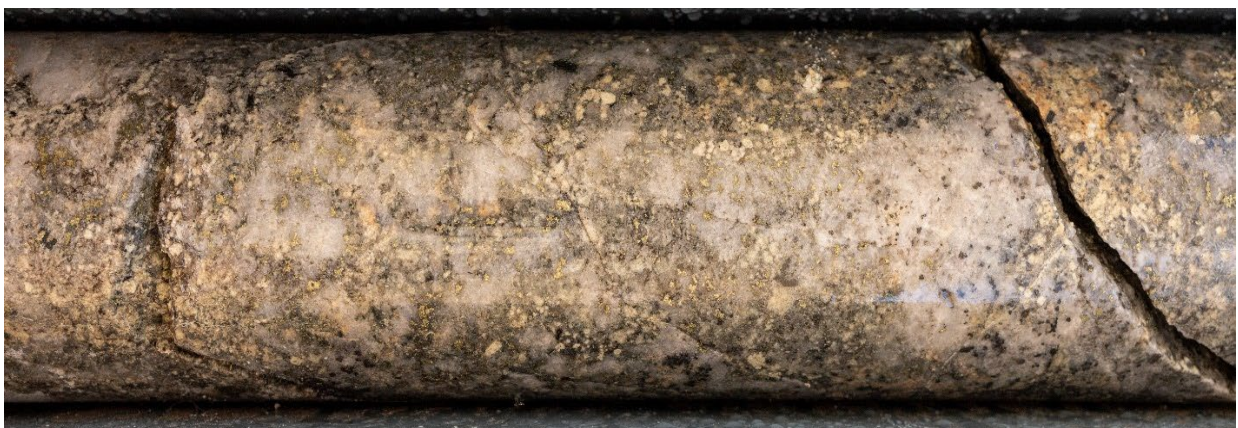
Figure 3. Altered granodiorite porphyry with silica flooding and disseminated chalcopyrite at 40.7m downhole depth in 25BRD0038. From within a 4.6m wide interval visually estimated to contain 2% chalcopyrite (0.70% Cu*). Core diameter 61mm.
