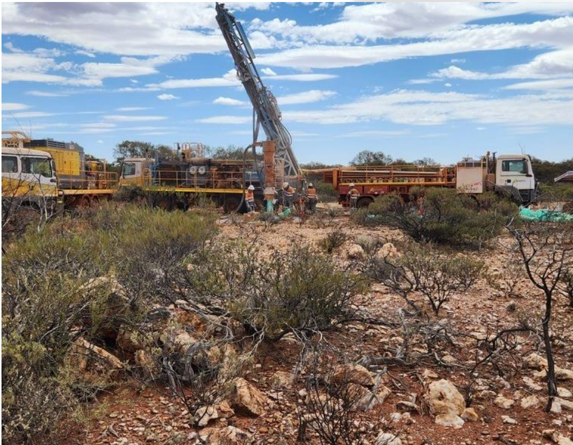
Figure 1: Ausdrill RC rig set up on the first Degruessa West drillhole testing soil anomalism. Quartz veining in Peak Hill Schist outcrop seen in foreground.
