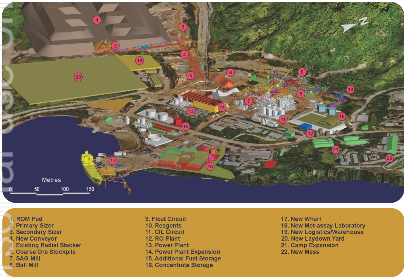
Figure 1: Simberi Expansion Project Process Plant Layout Design
