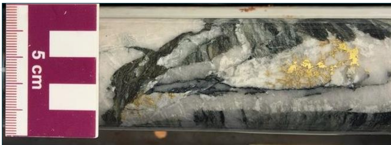
FIGURE 1: VISIBLE GOLD BETWEEN 503.52M AND 503.66M IN 25MBRCD002A
