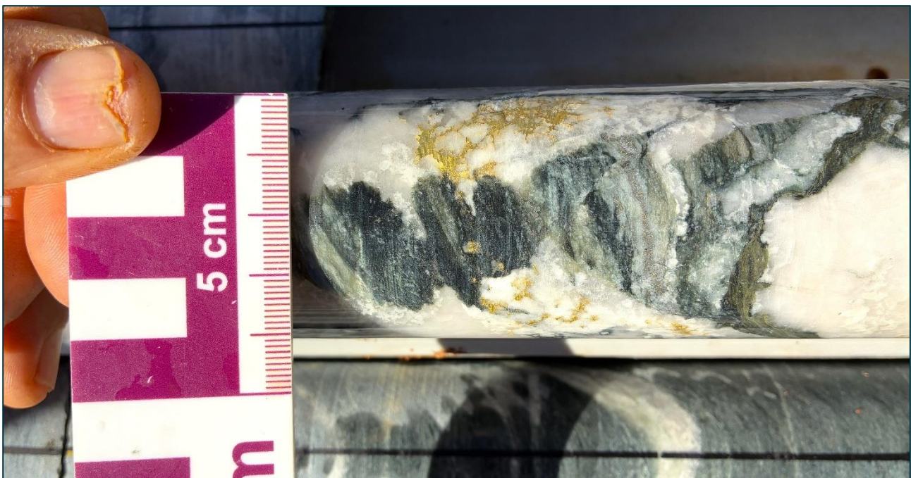
FIGURE 5: COARSE GOLD IS VISIBLE ON BOTH SIDES OF THE CORE IN 25MBRCD002A. VOLCANICLASTICS WITHIN THE BRECCIATED ZONE DISPLAY FINE DISSEMINATED PYRITE MINERALISATION WITH SILICA-SERICITE ALTERATION.
