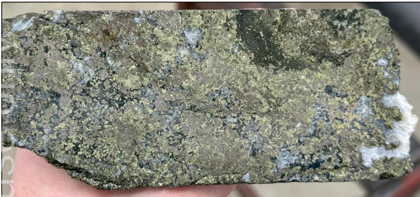
Figure 4. Core photograph from sample interval 169.6m to 171.6m in ZRSD25219, showing replacement style mineralisation with semi-massive chalcopyrite, pyrrhotite, pyrite and arsenopyrite assaying 0.3g/t Au, 3.4% Cu, 0.1% Zn, 27.1g/t Ag (6.8g/t AuEq).
