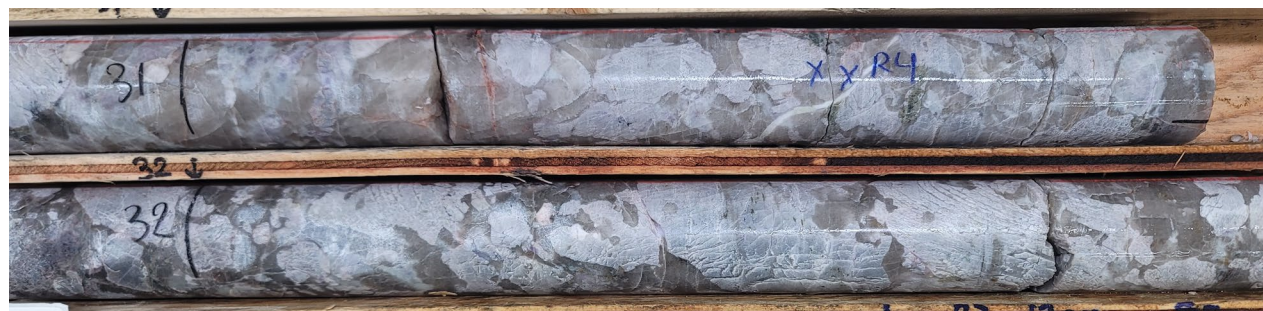
Figure 5: Large spodumene crystals in drill hole CV25-875 at ~32 m depth (core length) at the CV12 Pegmatite. Core graded 2.9 m at 2.70% \text{Li}_2\text{O} over sample interval (30.1 m to 33.0 m).
