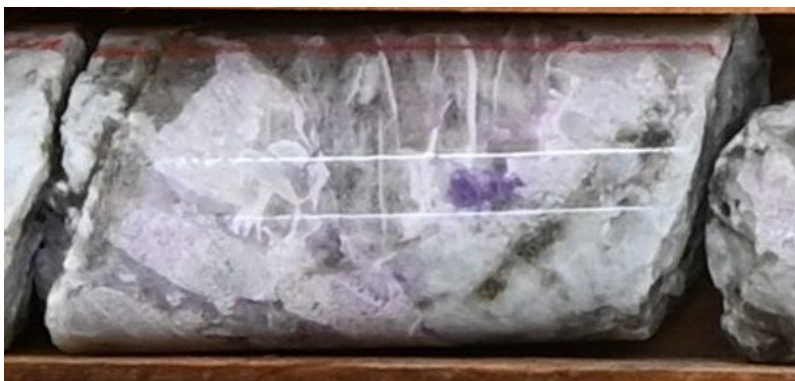
Figure 6: Large crystals of pollucite in drill hole CV25-880 at ~33 m depth (core length) at the CV12 Pegmatite. Core graded 1.5 m at 0.59% \text{Cs}_2\text{O} over sample interval (33.0 m to 34.5 m).
