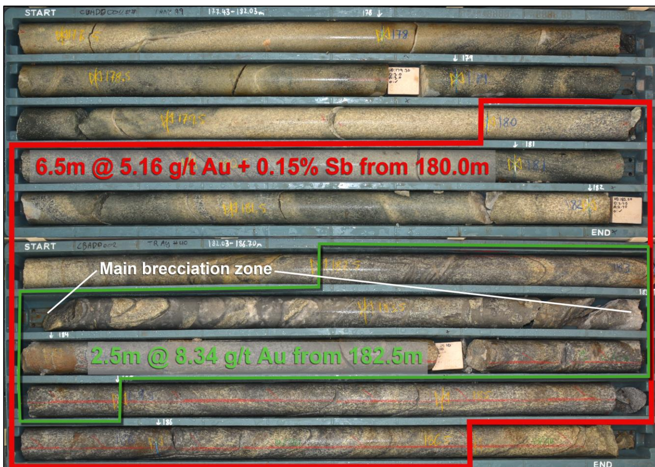
Figure 4: Core trays of CBADD002 highlighting the key thick gold zone and the main breccia zone.
