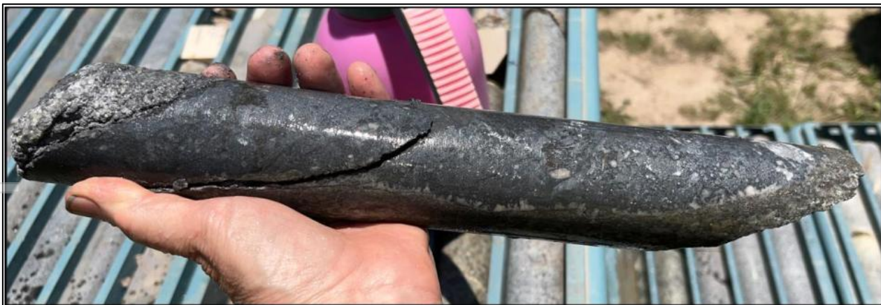
Figure 2 0.3m of quartz hosted massive stibnite* in hole CBADD007 from 139m.
