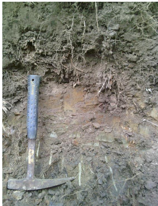
Figure 4: Soil profile investigations indicate conventional hand-auger sampling will be successful in this terrain (cross-sectional view, geopick for scale).
