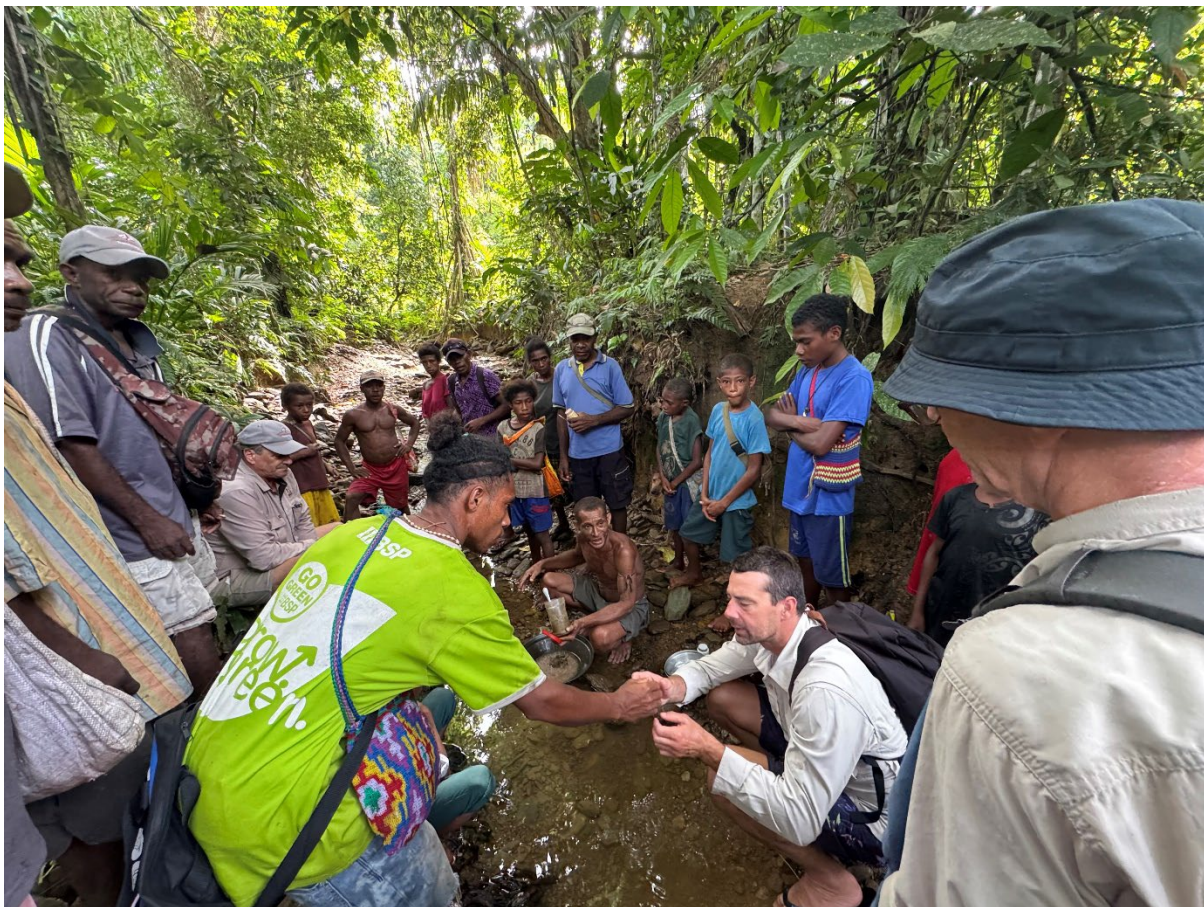
Figure 9: Gold panning at southern Wenasia area recovering fine grained alluvial gold from streams. (296820mE / 8891750mN (WGS84z56).
