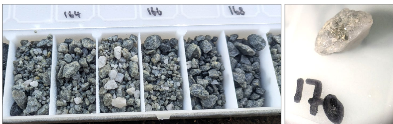
Figure 1. RC chips from SJRC003, highlighting a zone of strong sulphide alteration and quartz veining.
