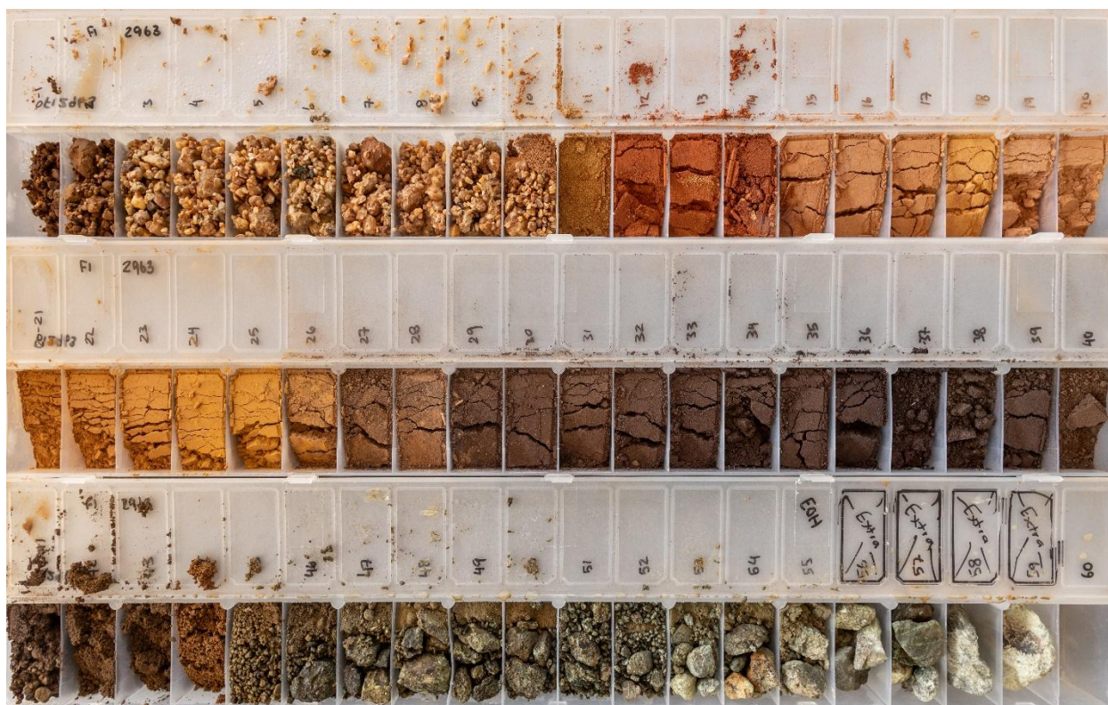
Figure 3b: Photograph of chip trays from FI2963 that was drilled at the Malamute Scandium Prospect. Each interval represents 1 metre of drilling.
