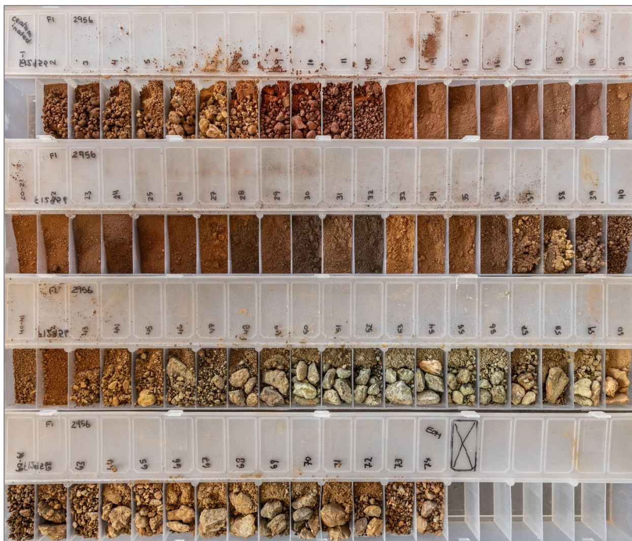
Figure 3a: Photograph of chip trays from FI2956 that was drilled at the Malamute Scandium Prospect. Each interval represents 1 metre of drilling.
