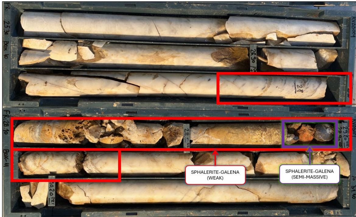
Figure 4: Drillhole KVDD001, drilling core from 25.3m to 31.1, PQ diameter
