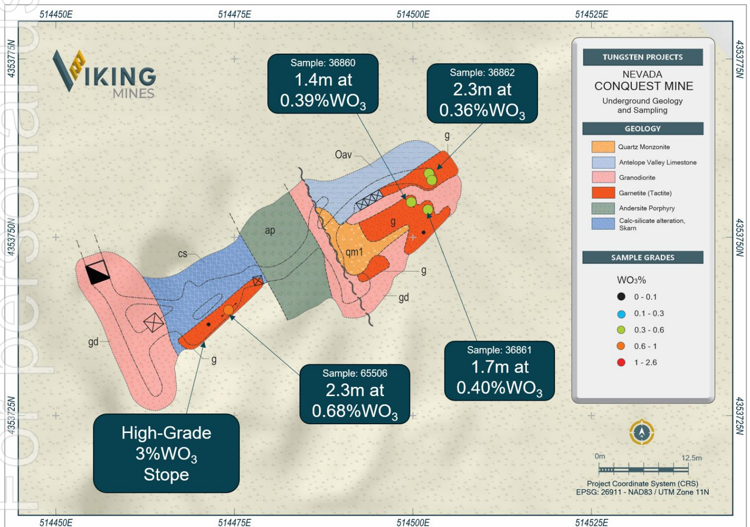
Figure 6; Underground geology map of the Linka-Conquest Mine showing location of high-grade 3%WO 3 stope and underground sampling results.
