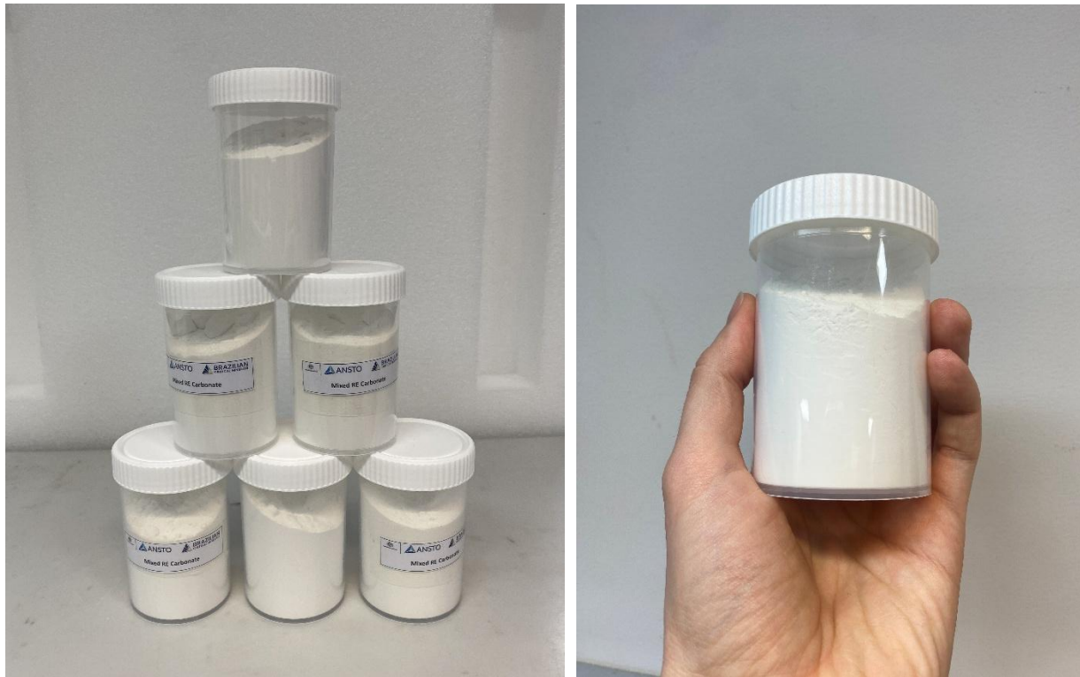
Figure 1. ANSTO produced MREC product containing on average approximately 52% by volume TREO (total rare earth oxides). Oxide samples ready for shipment to potential offtakers.
